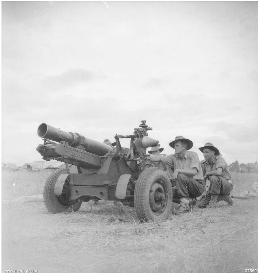
Fig.2: The short 25-pounder of the type utilised in the jungle campaign in Papua New Guinea and dropped into Nadzab on 5 September 1943 (Australian War Memorial photo AWM 075609)
