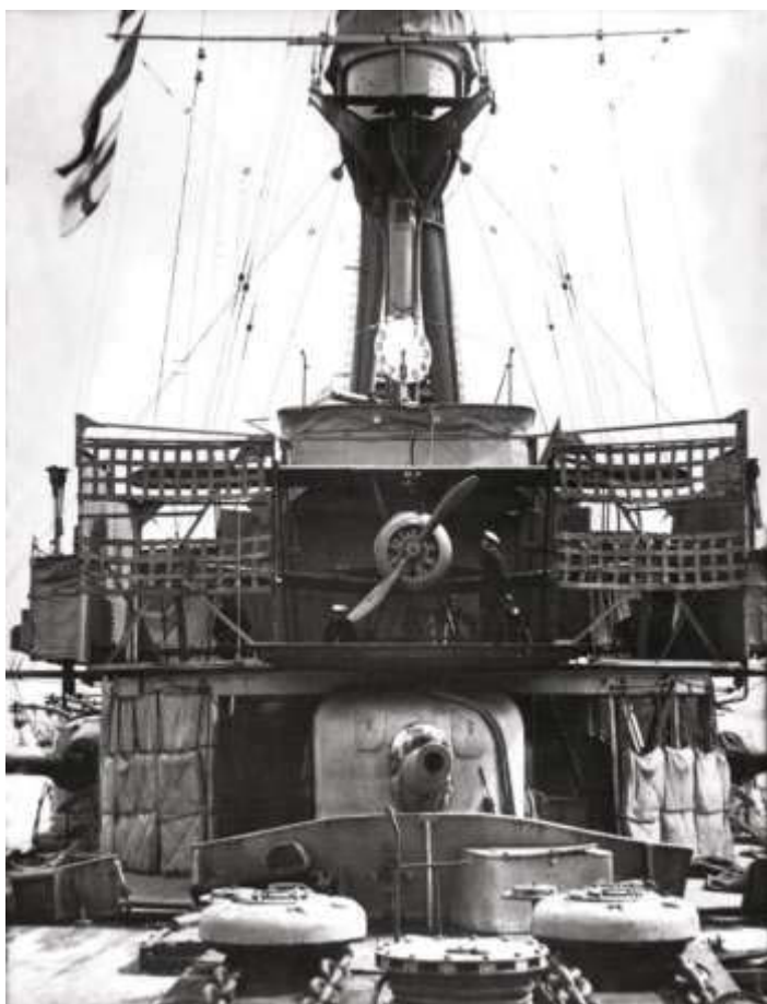
Fig.3: During the last year of the Great War, RAN ships operating in the North Sea all carried aircraft. HMAS Sydney and Melbourne launched their Sopwith Camel fighters from a flying-off deck mounted above the forward gun. (Sea Power Centre – Australia collection)
