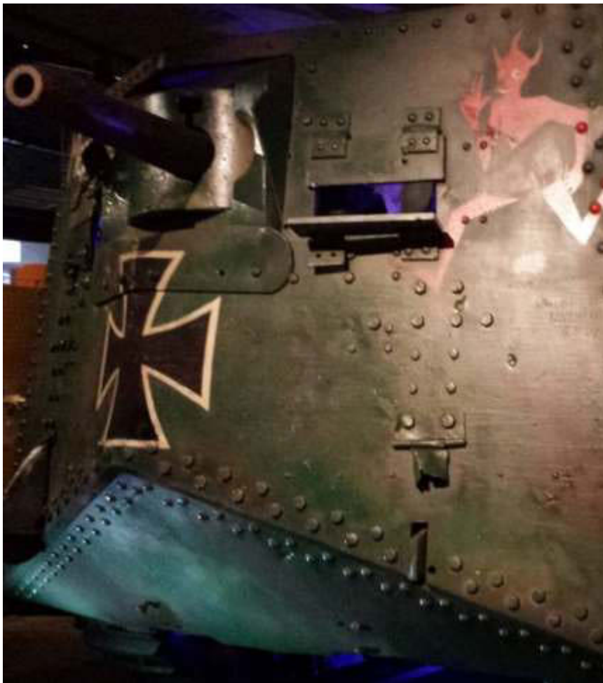
Fig.4 (left): A view of the bow or front end of 'Mephisto' showing the gun mount and some of the tank's markings. Note the damage to the mount from some attempt at demolition (author's photo)
