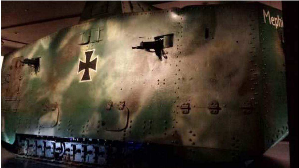
Fig.3 (above): A side view of 'Mephisto' showing the track and suspension and the riveted construction of the armoured plating (author's photo)
