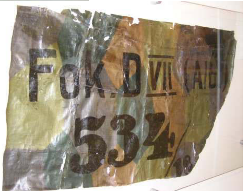
Fig.3 (below): Aircraft fabric souvenirs from France, 1918, by Lt Bruce Irvine. It is from a Fokker D.VII, the best of Germany's fighting scouts, and shows the aircraft's serial number, manufacturer (Albatros), and the distinctively printed 'lozenge' camouflage pattern. It was stored folded, and its identity hidden, until 2004. (Narromine Aviation Museum)
