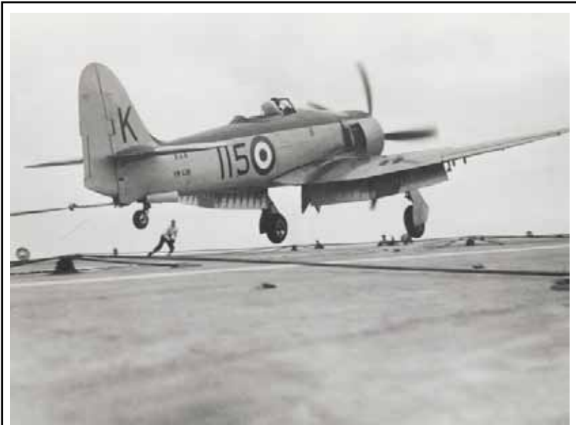
Photograph 4: Hawker Sea Fury landing on HMAS Sydney . Note the fully extended arrestor wire in the landing hook. Source: AWM 305450.
