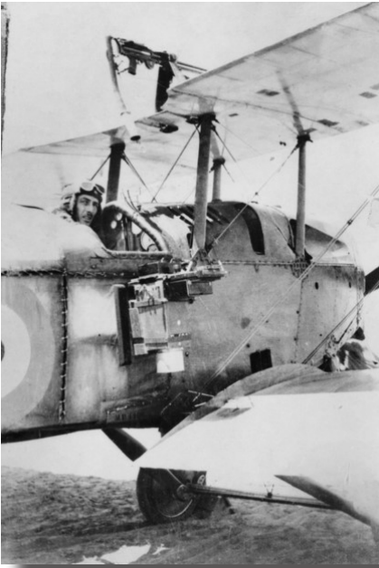
Figure 4: Capt (later AVM) Adrian Cole in a No.1 Sqn single-seat Martinsyde G.100 Elephant or 'Tinsyde'. A vertical Williamson camera is mounted on its fuselage side. Source: AWM P01034.038.
