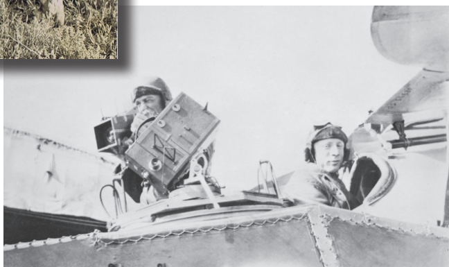
Figure 12: Captain Frank Hurley with camera and cinecamera in a Bristol Fighter piloted by Captain Ross Smith, February 1918. The guns have been removed and a camera platform fitted. Source: AWM P03137.010.
