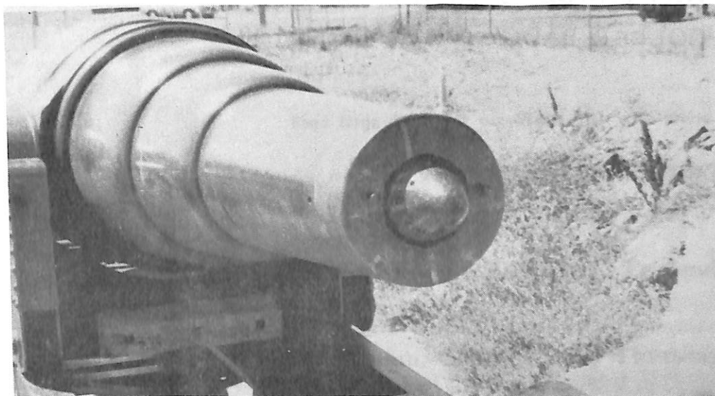
Close-up of muzzle of R.M.L. Armstrong 300 pounder at Fort Gellibrand, Williamstown A conical projectile is visible in the 10 inch barrel.
