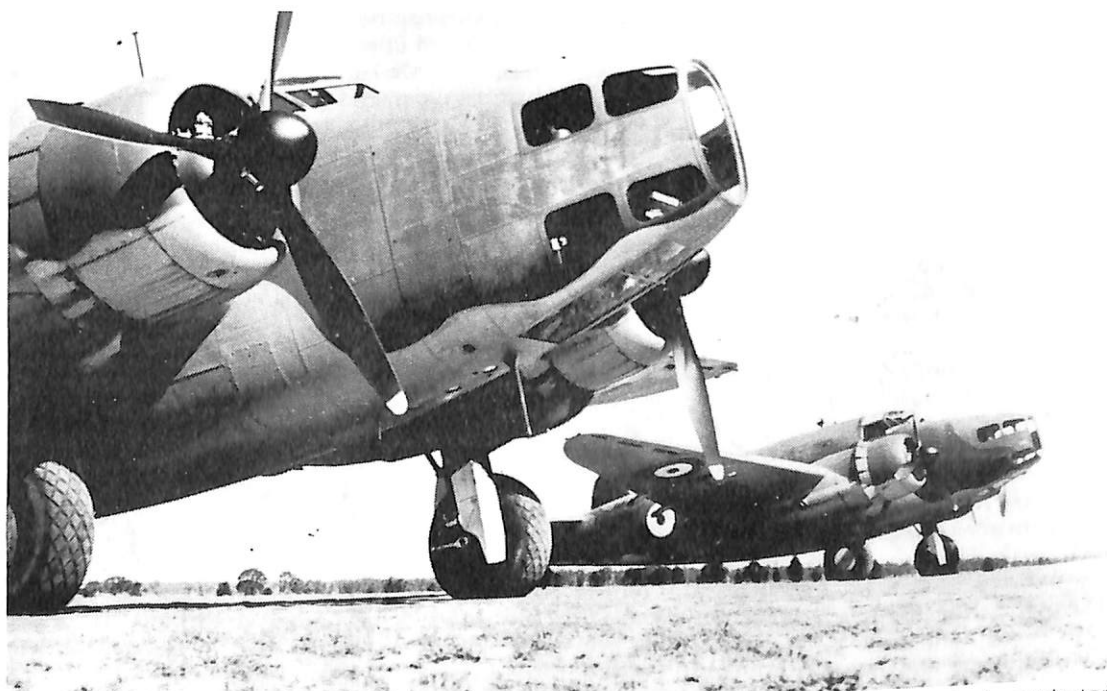
Early model Lockheed Hudson general reconnaissance bomber aircraft of the RAAF. The glazing in the navigator's position in the nose would have provided the author with a perfect view of the terrain. (AWM 128046)
