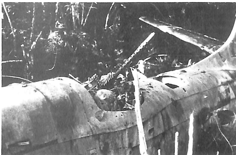
Rear gunner's compartment of Gloria showing 0.5-in. machine gun and ammunition. (Mike Claringbold)
