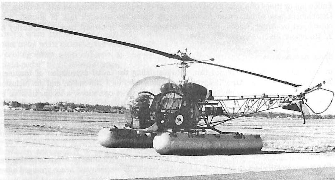
Bell 47G2A Al-672 photographed at RAAF Base Amberley in 1965. It is not fitted with platforms across its cross-tubes, as it was in West New Guinea in 1962. However, its radio configuration post-1962 is shown: the ARC 44 (FM) radio aerial extends diagonally at about a "one-o'clock" radial angle from the tail boom near the tail rotor, and the pair of ARC 44 homing aeriels (short, vertical) are further forward along the tail boom. AWM negative no. P01844.001
